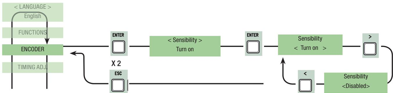
**Gate operation sensitivity:** this adjusts the obstacle detection sensitivity during opening and closing gate operation.
