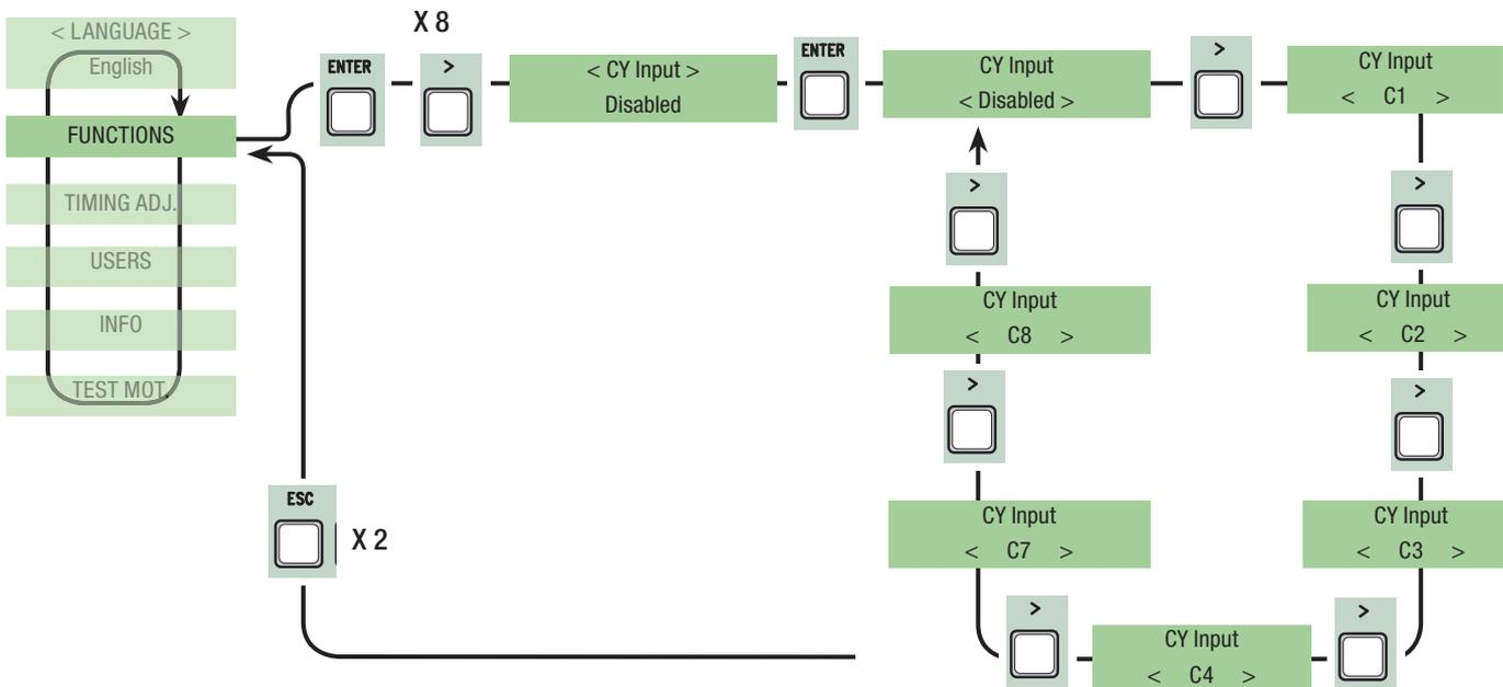
**CZ input:** safety contact input can take on the following functions: C1 (re-opening when closing), C2 (re-closing when opening), C3 (partial stop), C4 (obstacle stall), C7 (re-opening when closing, for sensitive edges), C8 (re-closing when opening, for sensitive edges) or, be deactivated. See safety devices on electrical connections.
