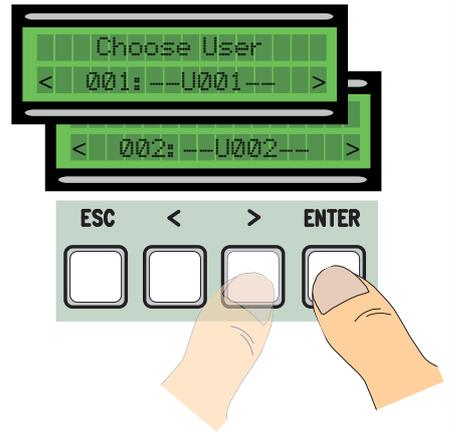
3) ... you will be asked to input a code. Send the code using the transmitter button or the slide-through card or the transponder.
