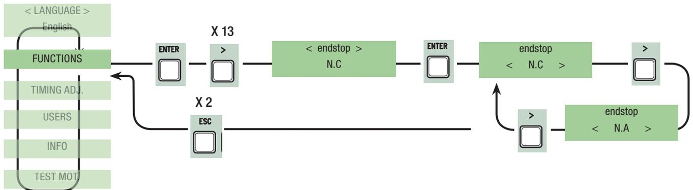
**Command 2-7:** setting the 2-7 contact to step-by-step mode (open-close) or sequential (open-stop-close-stop).
