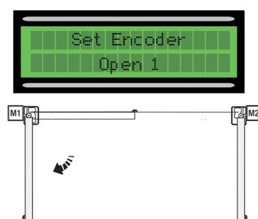
7) When the procedure is finished, the display will show "Set Encoder ok" for a few seconds.
