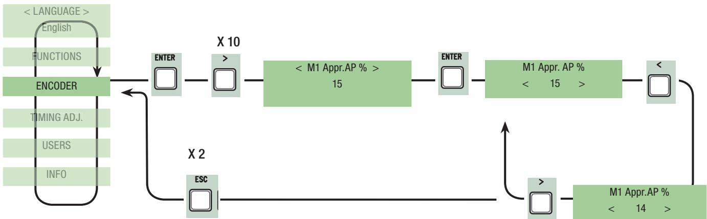
**M2 Opening approach %:** sets the point at which the gate begins adjusting deceleration before making contact with the opening endpoint of the second motor (M2).
