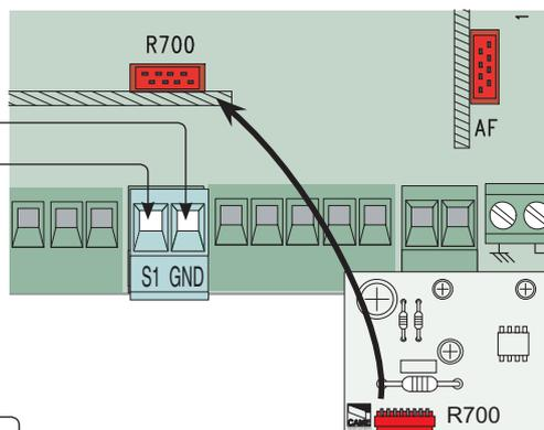
Stop button (N.C. contact) - Button to stop gate while excluding the automatic closing cycle. For movement to resume you must press the command button or transmitter button.
