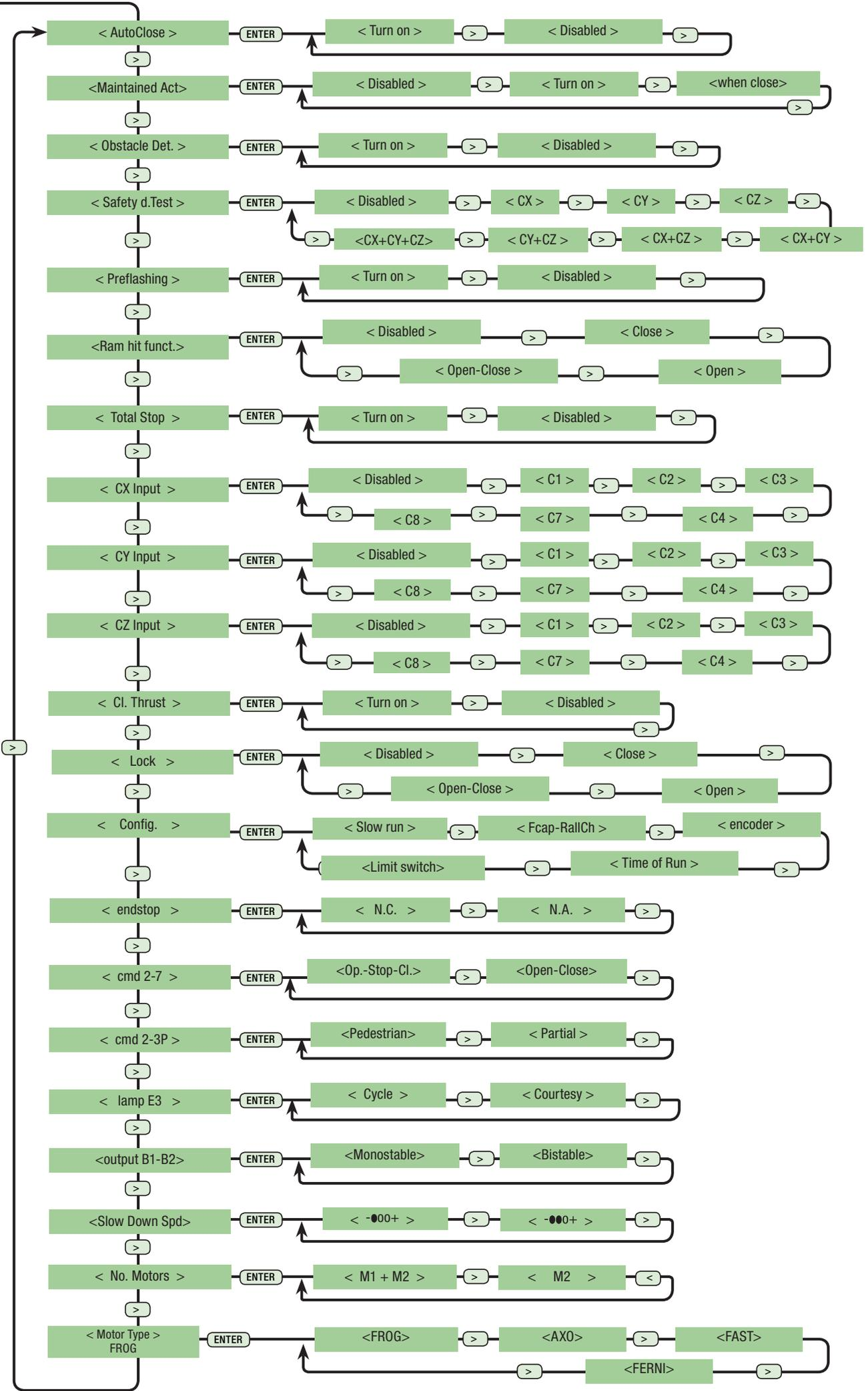
**Obstacle detected:** when motor is stopped (gate closed or after a total stop command) it prevents any movement if safety devices, such as photocells, detect any obstacles.
