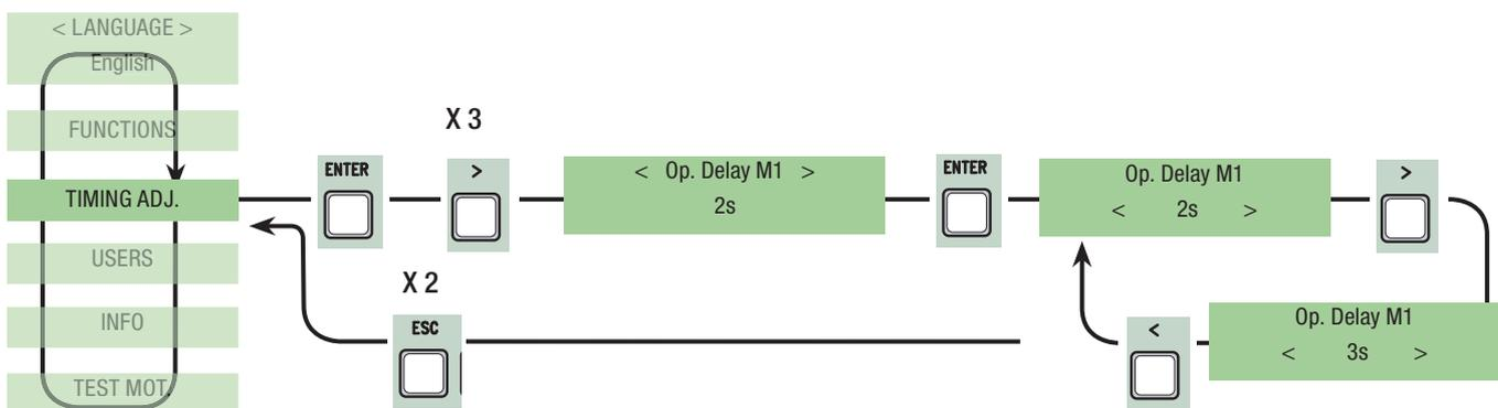
**M2 delayed closing:** the waiting time of the (M2) second gate leaf, unlike the (M1) first one, after each closing command. the waiting time can be set to between 0" and 60".
