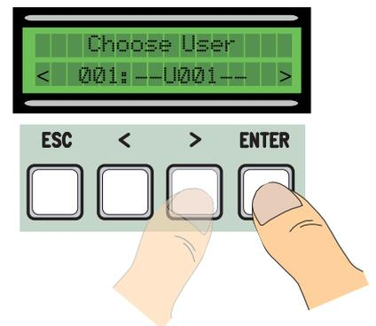
4) Confirm the text by pressing the ENTER key for a few seconds.
