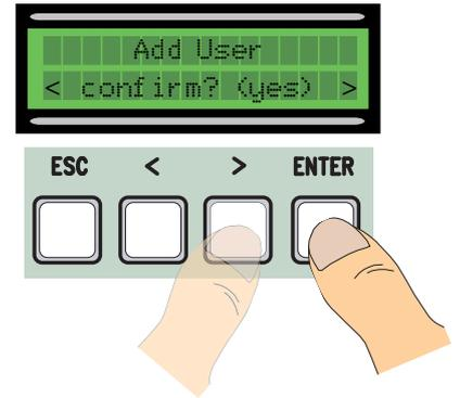
4) ... will ask to input a code. Send the code with the radio-command button or slide-through card or transponder.
