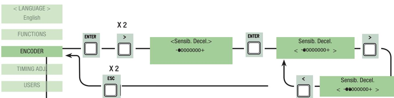
**Encoder Deceleration:** this activates the opening and closing deceleration starting points.
