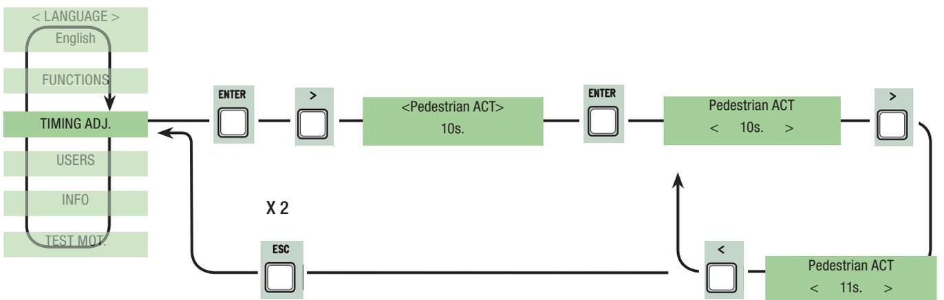
**Cycle time:** the working time of the motor during opening or closing phases is anywhere from 10" to 150".
