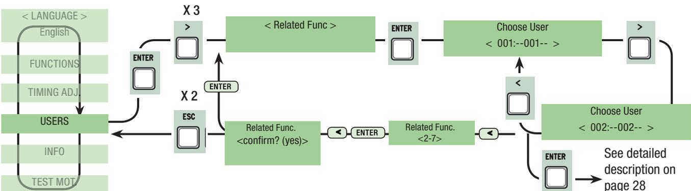
**Remove user:** to remove an existing user. Confirm the use you wish to remove with the ENTER key.
