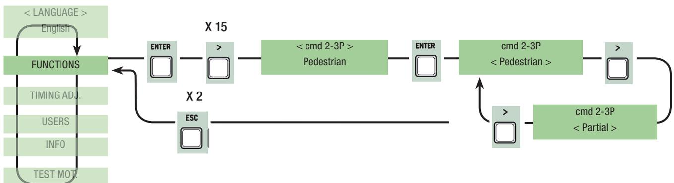
**E3 lamp:** configuring the lamp connected to E-E3:
