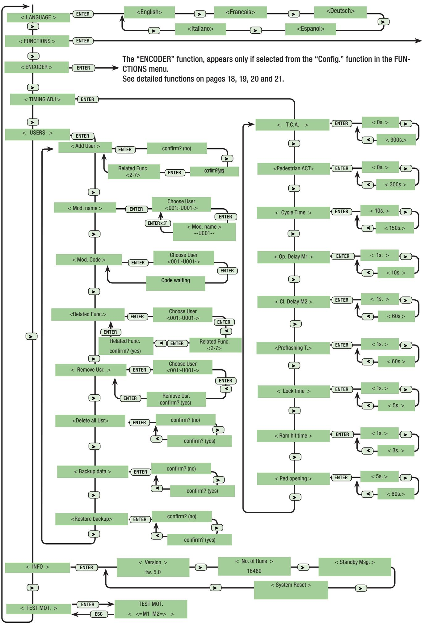
The "ENCODER" function, appears only if selected from the "Config." function in the FUNCTIONS menu.
