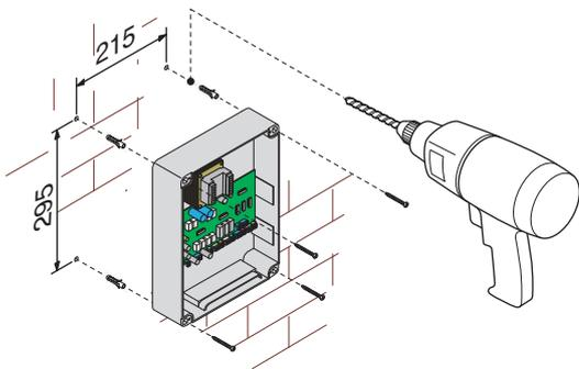
2) Perforate the pre-punched holes and insert the cable glands with the corrugated tubing for the electrical cables to travel through.
