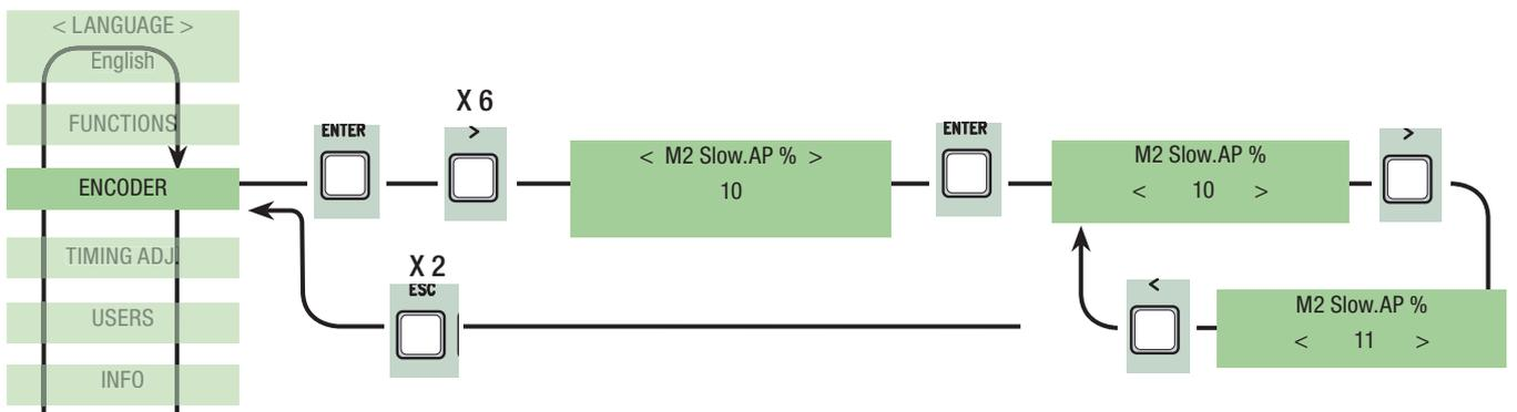
**M2 closing deceleration %:** this adjusts the (M2) second motor's deceleration starting point before the closing endpoint. The deceleration starting point is calculated as a percentage (from 1% to 40% of a full gate run). See illustration on page 28. N.B.: this function appears only if it is activated in the "decel. Enc" function in the ENCODER menu.
