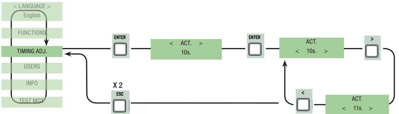
**Automatic Pedestrian Closing:** waiting time of the (M2) second gate leaf when in the open position. Once this time interval has elapsed, the gate automatically closes. The waiting time interval can go anywhere from 0" to 300".
