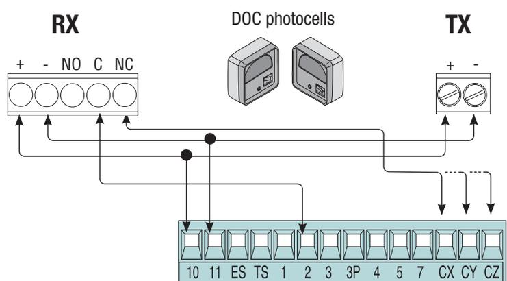
Configure either (N.C.) contacts CX, CY or CZ, input for EN 12978 compliant safety devices such as sensitive edges. See CX input functions in:
