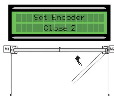
5) ...then, the gate leaf of the second motor, will perform an opening run until fully open...
