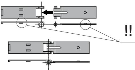
4) Insert the pressure hinges into the box (on the left or right as you wish) and set them using the provided screws and washers.
