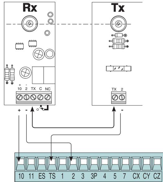
At each opening and closing command, the control board assesses the efficiency status of the control devices (photocells). Any anomaly found is signalled with the flashing of the LED on the control panel. Consequently it cancels any commands coming from the remote control or the button.
