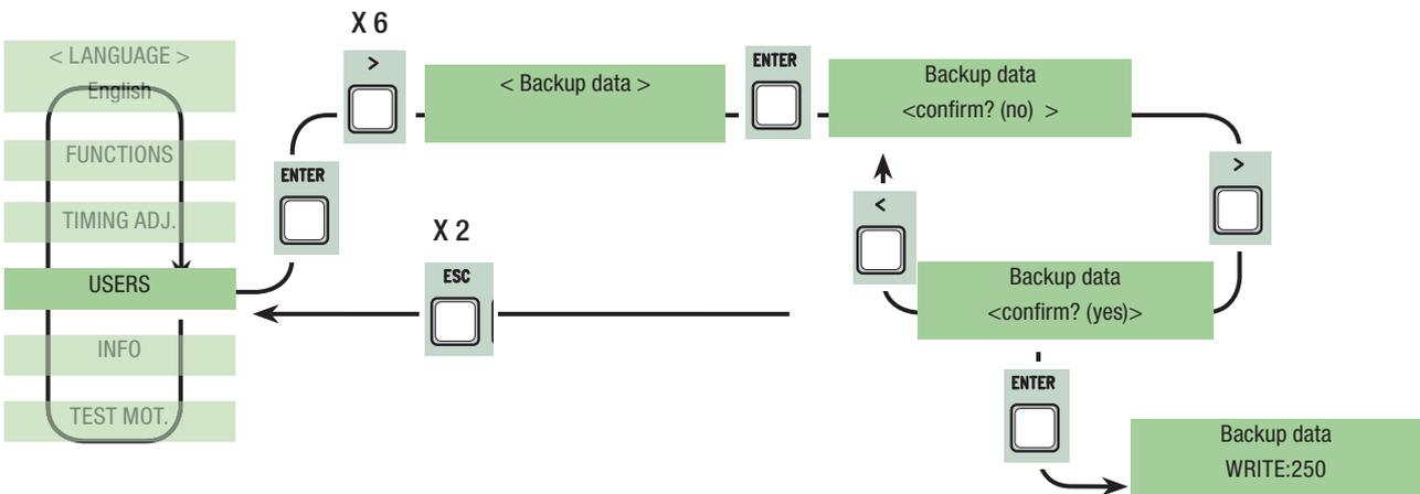
**Restore backup:** to load the data saved on the memory roll onto card (if the card is of the same version it loads both users and settings, otherwise it only loads the users).
