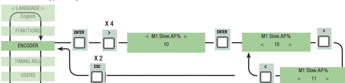
**M1 closing deceleration%:** this adjusts the (M1) first motor's deceleration starting point before the closing endpoint. The deceleration starting point is calculated as a percentage (from 1% to 40% of a full gate run). See illustration on page 28. N.B.: this function appears only if it is activated in the "decel. Enc" function in the ENCODER menu.
