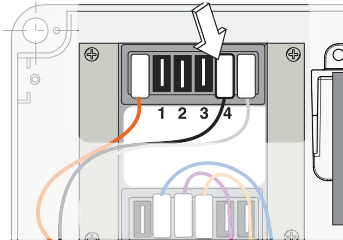
To vary the motor torque, move the shown faston (the one with the black wire) to one of the 4 positions:
