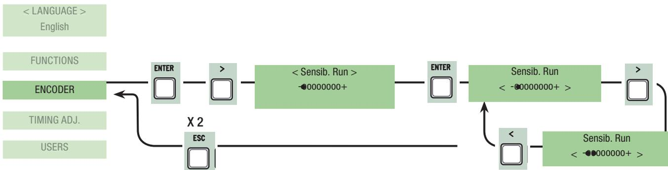
**Deceleration sensitivity:** it adjusts the obstacle detection sensitivity during opening and closing gate deceleration.
