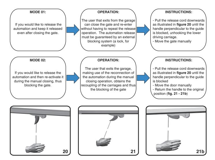
① During manual operation use only the door for opening and closing, thus avoiding strain on the carriage by pulling the release cord.
